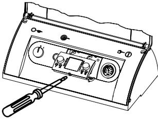
2. Remove the BM programming module from the boiler control unit.
