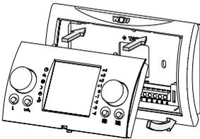
3. Click the BM programming module into the wall mounting base.
