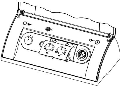
4. Click the facia into the front. Then push the rotary selector for DHW and the rotary selector for central heating with pointers set to 5 onto their respective shafts. Then carefully turn the rotary selector fully anti-clockwise and then clockwise. If the rotary selector cannot be turned fully clockwise and anti-clockwise, pull the rotary selector off again and turn it 180°.
